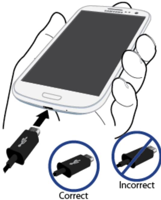
3. Plug the AC adapter into an electrical outlet and charge your battery. Fully charging a battery may take up to three hours.
